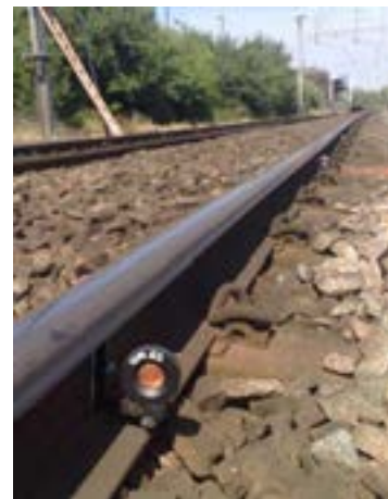
Pictured above: One of the 300 mini prisms fixed to the rails to monitor the track.
